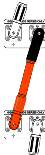
High voltage Series connection
