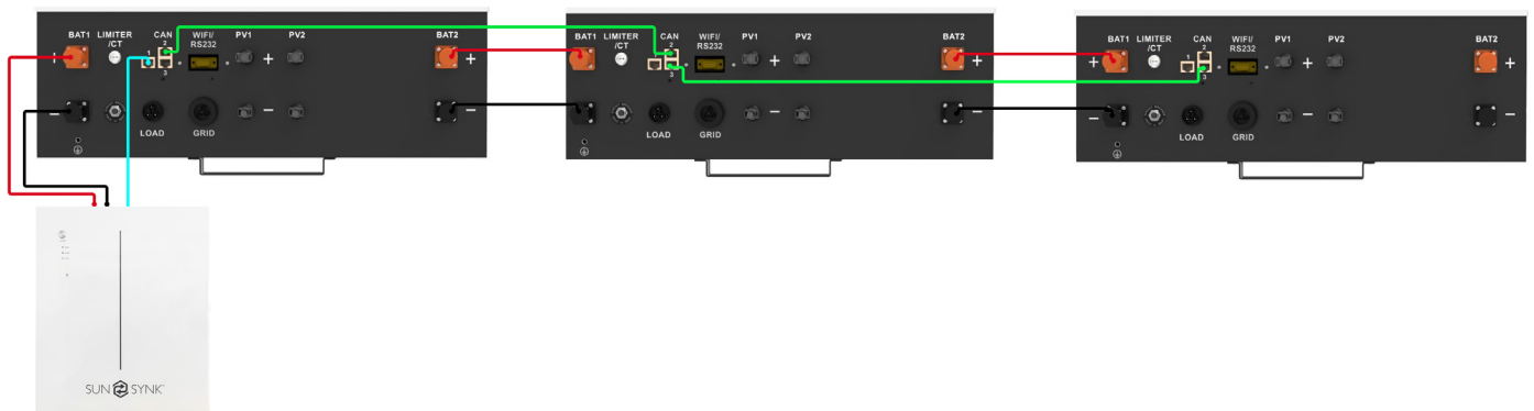
Inverter Unit: 3 External Battery Number: 1
