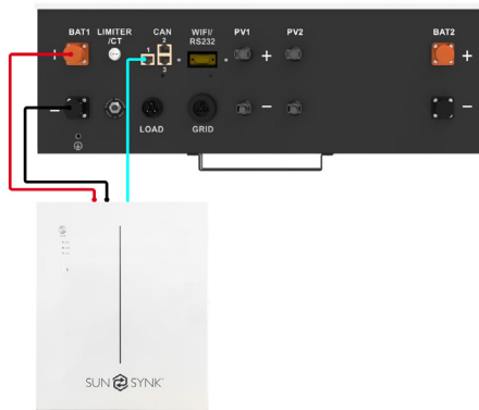
Inverter Unit: 2 External Battery Number: 1
